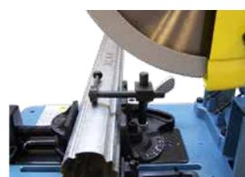
**Système de fixation excentrique**
