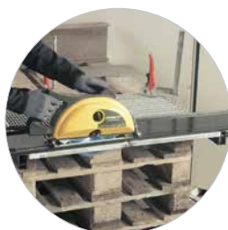
Ideal for cutting metal grids with LBS saw blade
