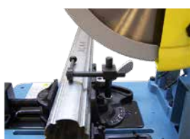
Excentric clamping system
