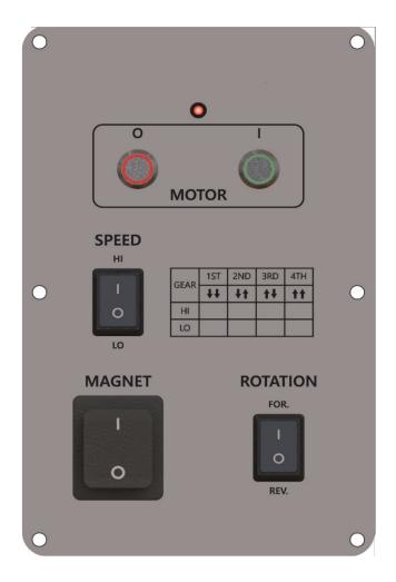
① MAGNET SWITCH: Main switch of Machine
