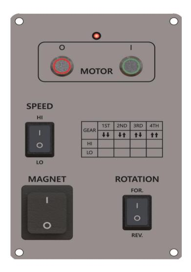
① MAGNET SWITCH: Main switch of Machine
