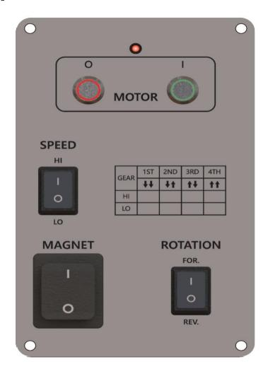
① MAGNET SWITCH: Main switch of Machine
